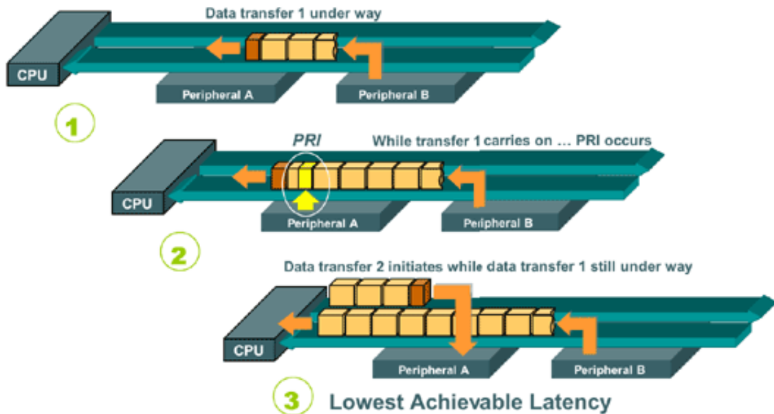
Figure 11 – HyperTransport Priority Request Interleaving natively provides a mechanism that enables the insertion of commands within lower priority data traffic so that higher priority traffic can be initiated concurrently.
