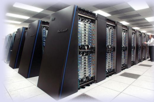
Blue Gene/P Peta-Scale Supercomputer 73,728 Nodes Scalable to 221,184 Nodes
