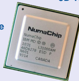
NumaChip™ Scalable, Cache Coherent, Shared Memory 3D Torus Interconnect Controller Chip
