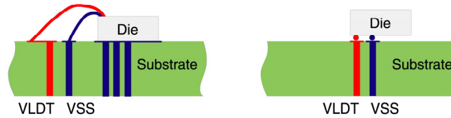
Figure 41. Differences in VLDT Interconnect for Wirebond and Flip-Chip Technologies
